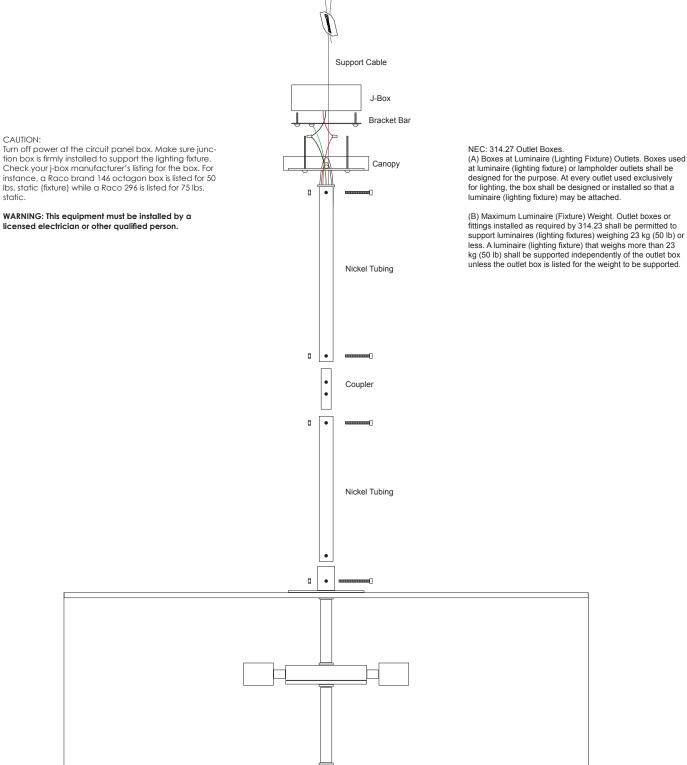
tion box is firmly installed to support the lighting fixture. Check your j-box manufacturer's listing for the box. For instance, a Raco brand 146 octagon box is listed for 50 lbs. static (fixture) while a Raco 296 is listed for 75 lbs. static.
